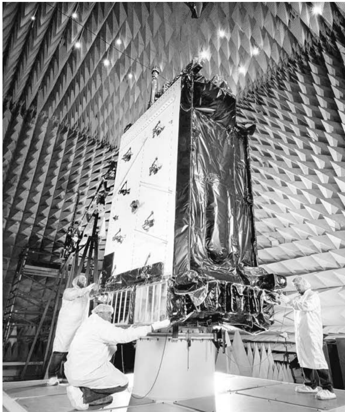
This March 22, 2016, photo provided by Lockheed Martin shows the first GPS III satellite inside the anechoic test facility at Lockheed Martin's complex south of Denver.
